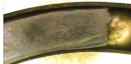
Damaged Bearing 20x
